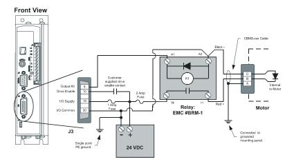
Figure 17: Epsilon Brake Wiring Diagram using the I/O Connector
